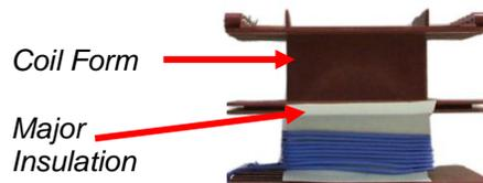
Coil Form (bobbin) with Major Insulation between Winding Wire and Coil Form
