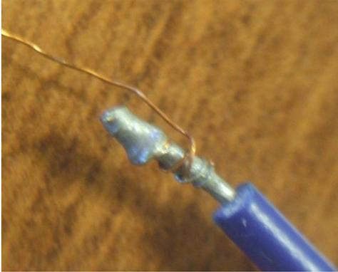
*Coil Wire Connected to Connecting Cables*
