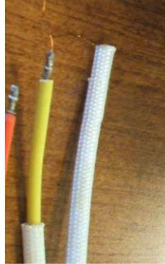
*Sleeving before covering junction and Sleeving after covering junction*
