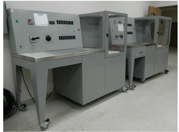
*Two of the many high-voltage test apparatus designed, fabricated, calibrated and maintained at ELTEK Labs.*
