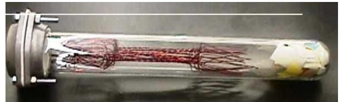
The standard Sealed Tube Vessel loaded with twisted pairs of copper wire and electrical insulation materials
