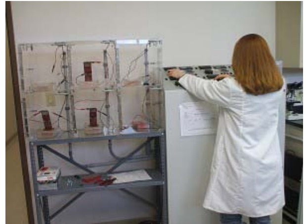
Lab technician Corina Wenzara, of Eltek International Laboratories in St. Charles, performs inclined plane testing, which is a continuous containment flow across the surface of any material with a specified voltage applied. Eltek recently was recognized as an internationally accredited laboratory.
