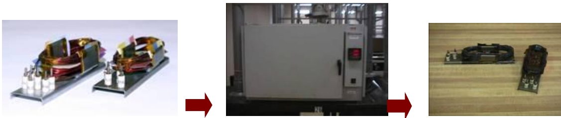
Photos showing decomposition due to heat exposure of EIS test specimens.
